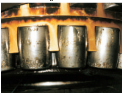
Wear on roller elements
