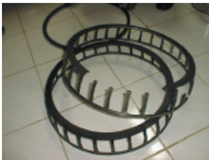
Failure of cages
