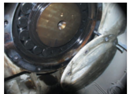
Pittings on the inner ring of a bearing
